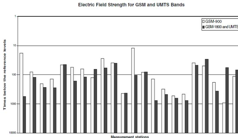
Figure 4. Measurement results for the downlink radiation of base stations in Greece [44].
