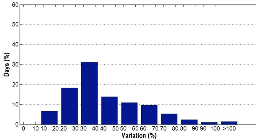
**Figure 7.** PDF of the variation between maximum and minimum electric field strength values from 60 stations in the monitoring network in Greece [53].
