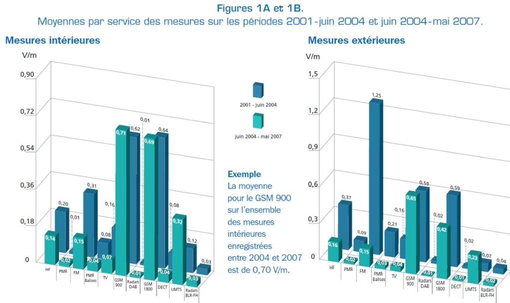
**Figure 1.** Mean values of electric field strength measured in France [42].
